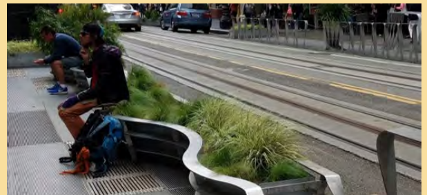
W3: Example of stormwater planter to be used along Bay Trail
