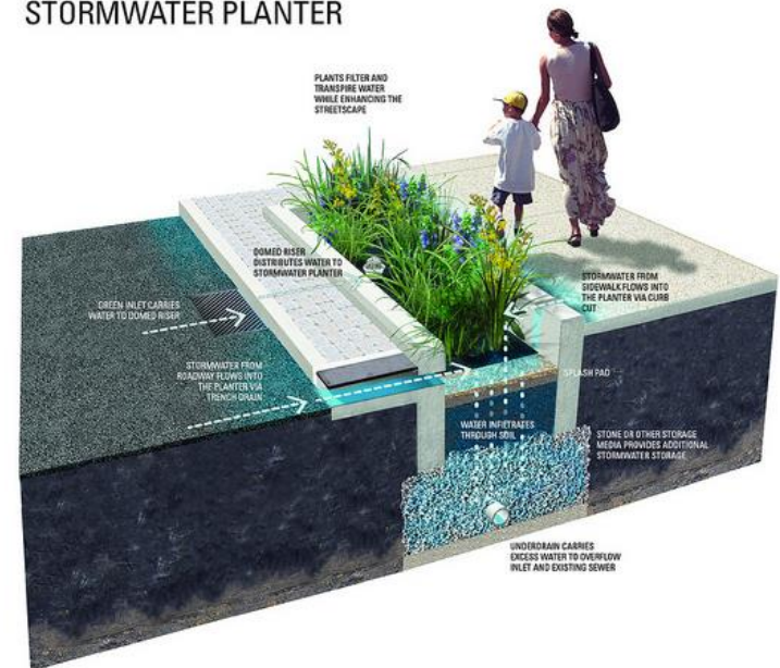
Stormwater planter cleans water from roads before reaching creeks
