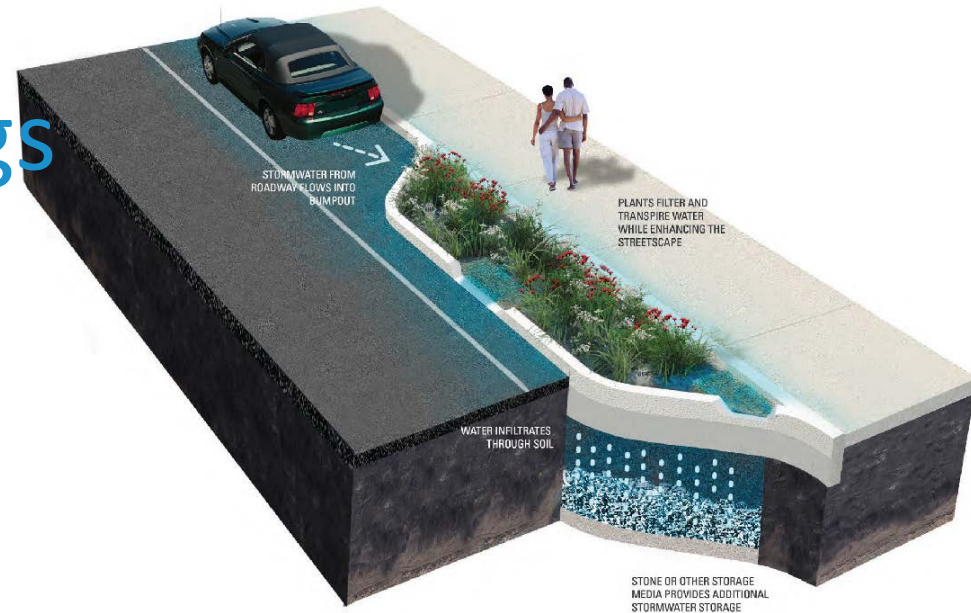
Mid-block Stormwater Bump-out
