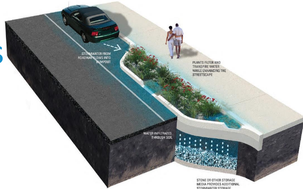
Mid-block Stormwater Bump-out
