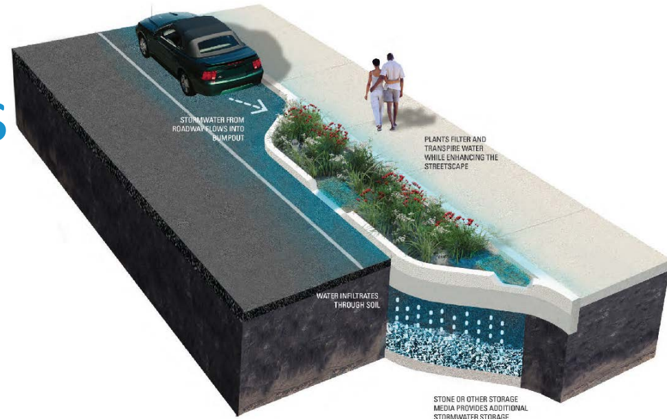
Mid-block Stormwater Bump-out
