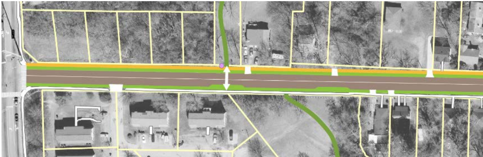
Example of a street that integrates planted swale and sidewalks within 50 ft right-of-way.
