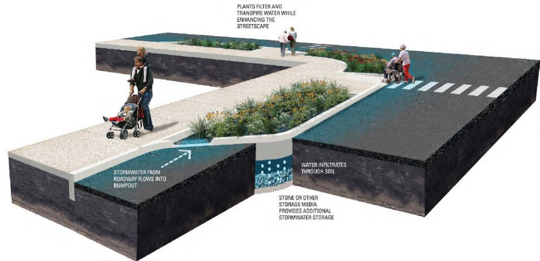
Corner Stormwater Bump-out
